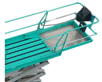
Manual deck extension of 51" 770 lb / 550 lb Capacity Number of Occupants - 3 / 2
